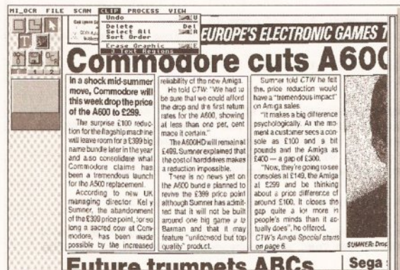
The next step is to draw clip boxes around the three text areas to be OCRed
